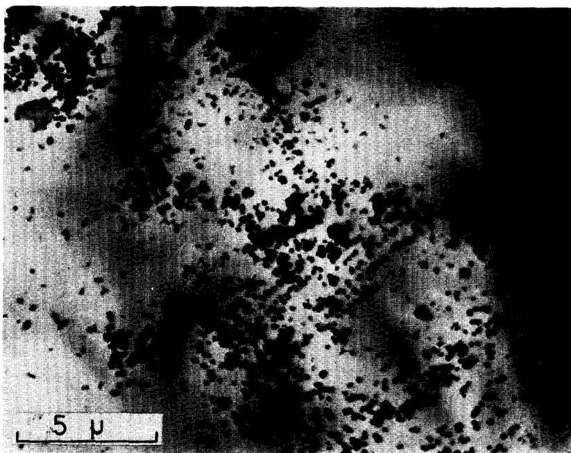
FIG. 3. Electron-microscope autoradiograph of tritium on nickel plate.
